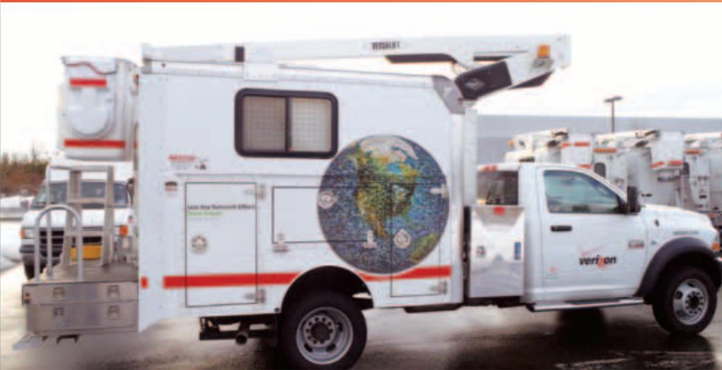
*By 2015, 15% of our fleet will be alternative-fuel vehicles such as this “worksite hybrid.” The lithium ion batteries on this vehicle power the lift, air conditioning and all other utility features.*
