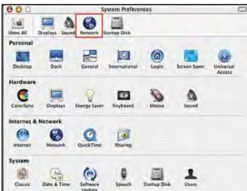
**Step 3** The Network window opens. Select Built-in Ethernet in the show field. Select Manually in the Configure IPv4 field.
