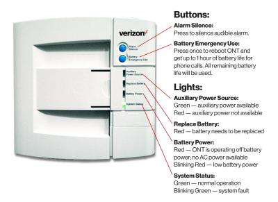
Note: The optional battery backup unit does not supply backup power to all voice services. VoIP and Business Digital Voice cannot not be powered by the battery backup. Not all battery backup units look identical to the image shown above.
