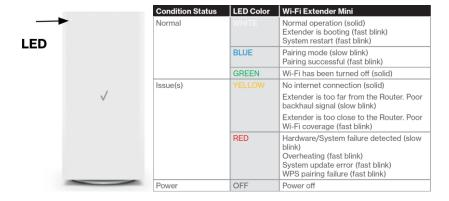
The status LED will be on white and solid when your Verizon Wi-Fi Extender is turned on, connected to the Internet, and functioning normally. Refer to the chart above for additional details.
