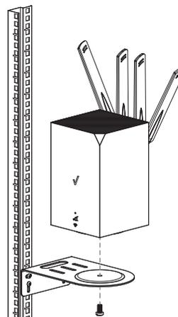
2. Mount the device on the bracket and secure it with the supplied screw.
