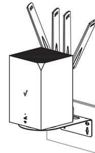
5. Ensure the device is firmly secured to the bracket.
