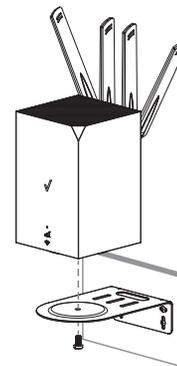
4. Mount the device on the bracket and secure it with the supplied screw.
