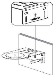
1. By following the "THIS SIDE UP" direction, align the bracket with the wall. Draw the screw installation points.
