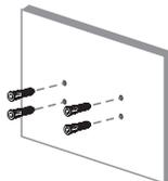
2. Drill the holes and place the four (4) anchors.
