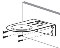
3. Align the bracket with the wall anchors and secure four (4) screws through the bracket holes and into the wall anchors.
