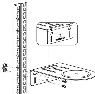
1. By following the "THIS SIDE UP" direction, secure the bracket to the rack with mounting screws (not supplied).
