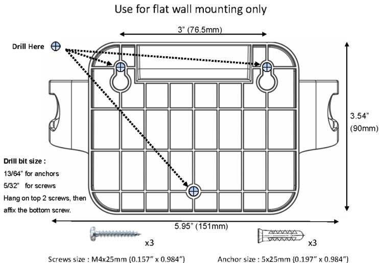
3. Drive two screws into the wall. Leave the screws extended about 0.2 inches from the wall.
