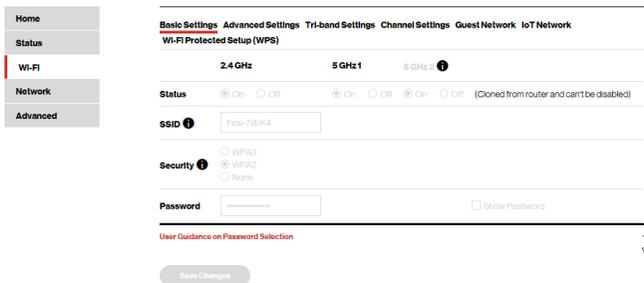
*To view the basic radio, SSID and security settings:*
