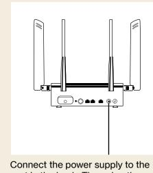
port in the back. Then plug the Internet Gateway into an outlet.
