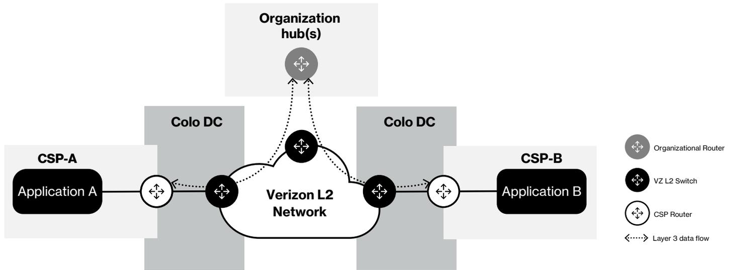
In this case, the Layer 3 operations (BGP routing) are established between the organization routers and the CSP routers directly, with the WAN only providing a medium to connect the two. It is then the organization’s responsibility to manage the BGP sessions with the CSPs and also to route traffic between the different applications.
