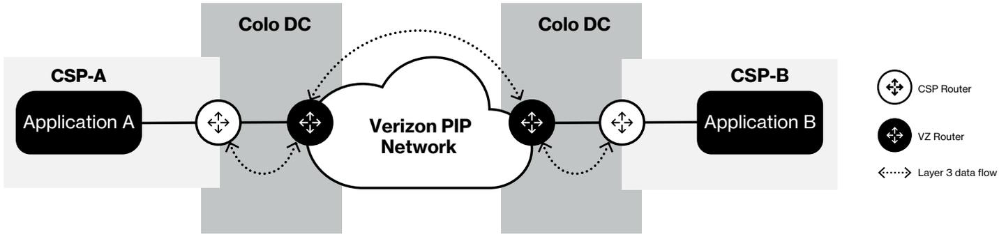
**At numerous data center co-locations, Verizon has deployed physical routers (typically two for redundancy) and established physical cross connects to a large number of CSPs. When a connection is required to a given CSP, a virtual port is configured on the aforementioned routers which is used to connect the CSP hosted applications to Verizon backbone network. Standard IP routing is then used to exchange data between the different routers.**
