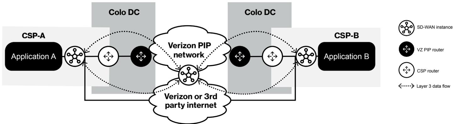
**The challenge with this design is the availability of SD-WAN virtual instances with the different CSPs. While the support of those instances in AWS and Azure is common, it is less so with other smaller and more specialized CSPs. Verizon supports this design with Cisco and Versa for the SD-WAN with a small number of CSPs. Connection to the Verizon Private IP network is done through Secure Cloud Interconnect, Software Defined Interconnect or dedicated Private IP port.**
