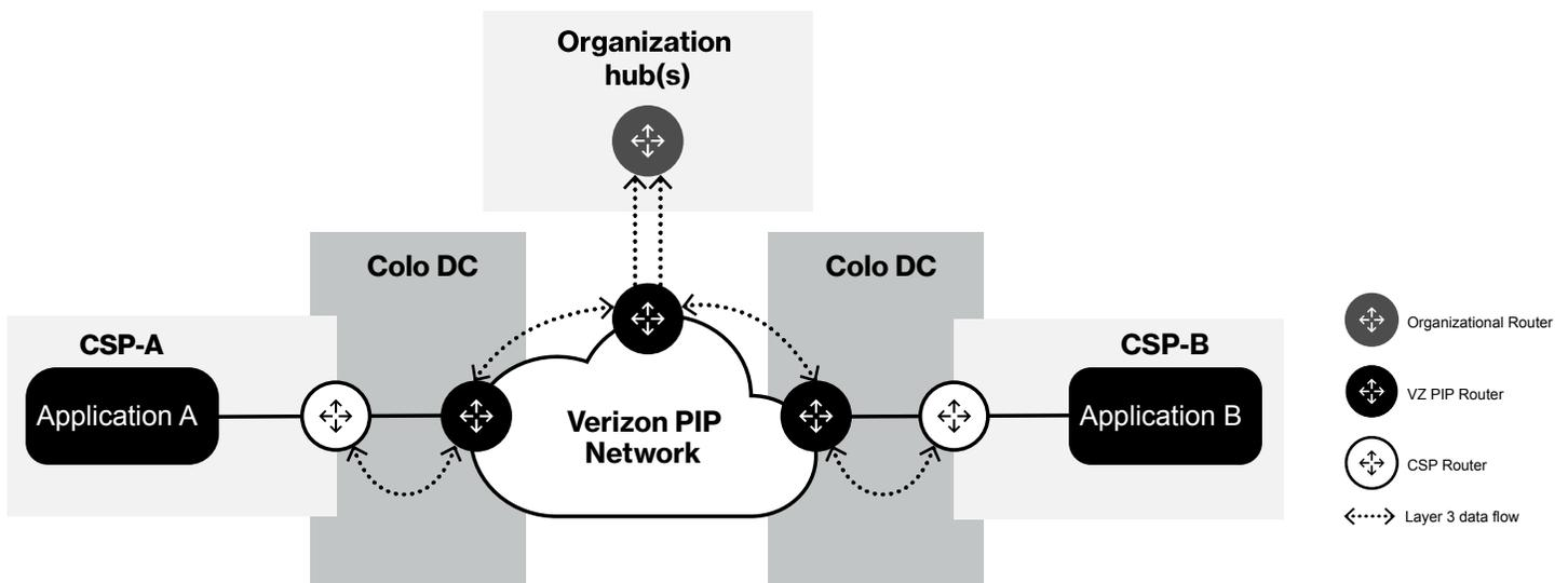
**With the Layer 3 option, Verizon manages the BGP sessions between the Private IP network and the CSPs from one side as well as between the Verizon Private IP routers and the organization routers from the other side. Standard routing protocols are used to route traffic from the CSP routers to Verizon routers, between Verizon routers and then to the organization router(s) and back.**
