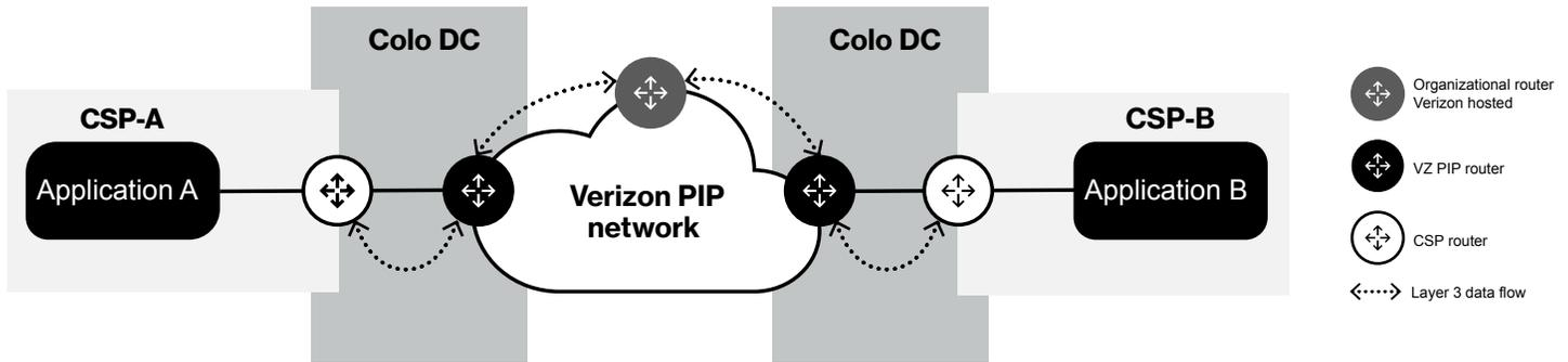
**This design is supported with Verizon services such as the Secure Cloud Interconnect, Software Defined Interconnect or a Dedicated Private IP Port which are used to connect the CSP hosted applications to the Verizon Private IP network and from there to the Verizon hosted router(s).**
