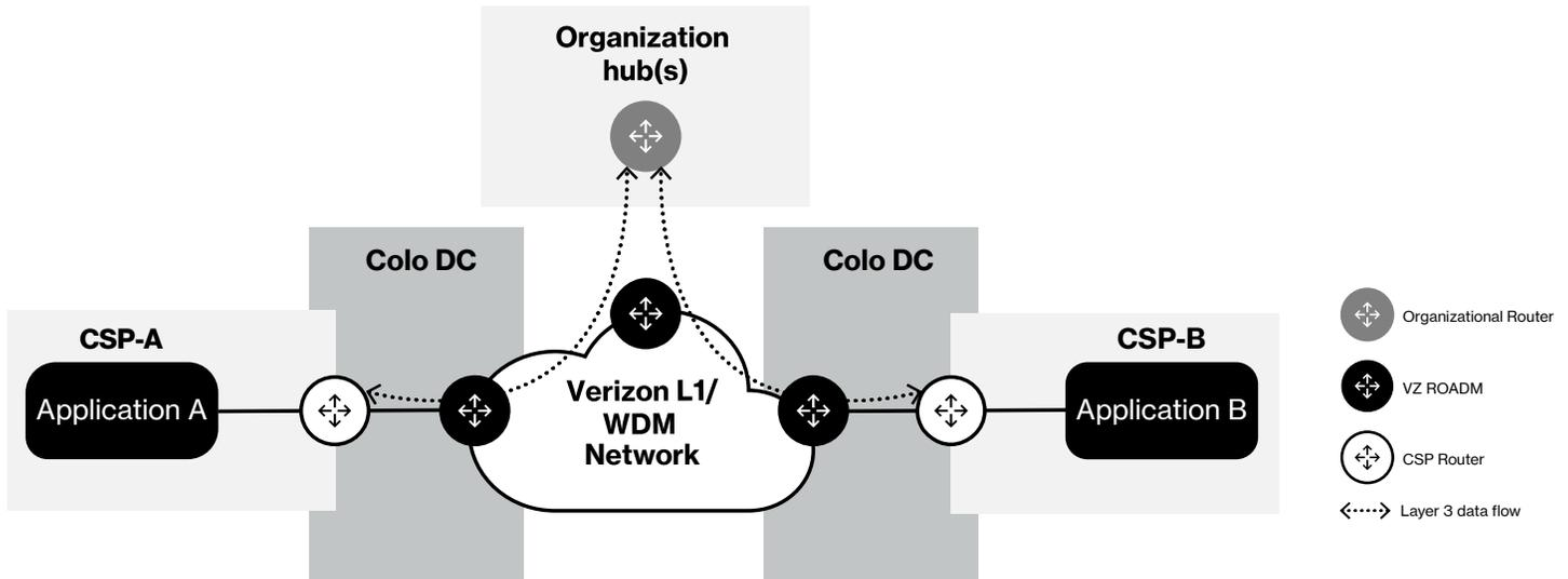
**Like with the ELINE design, the Layer 3 operations (BGP routing) are established between the organization routers and the CSP routers directly, with the WAN just providing a medium to connect the two. The BGP sessions as well as routing between the applications is also managed directly by the organization.**
