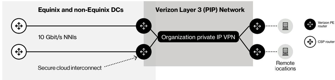
**To connect an organization to a CSP that is part of the SCI network, an SCI port is (software) configured for that purpose on the Verizon colocated routers. The SCI port is then attached to the organization's Private IP VPN on one side and to the CSP routers on the other side. The SCI port runs the required BGP session with the CSP routers. The logical SCI port is then used to route traffic between the two entities.**
