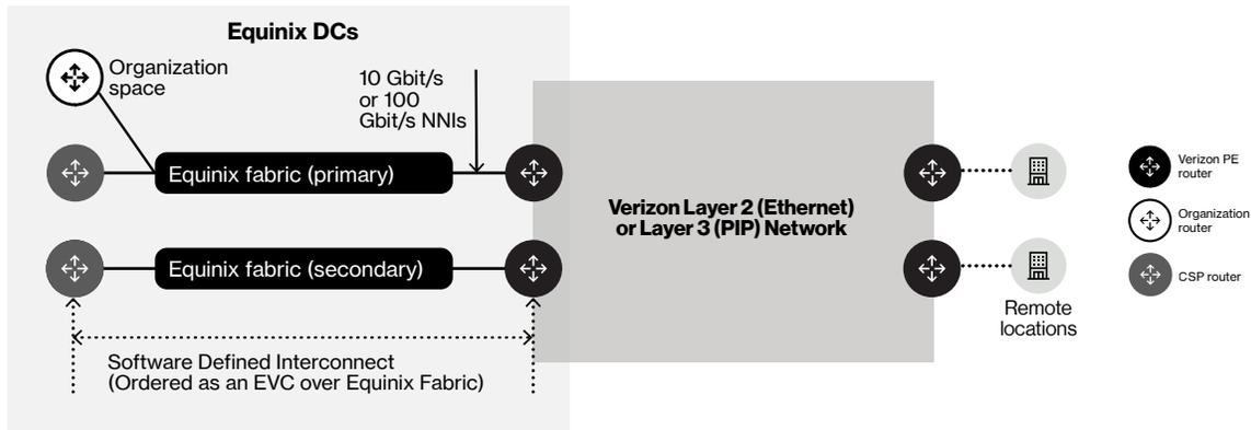
**When an organization wants to connect to a CSP with Software Defined Interconnect, an SDI access is (software) configured on the Verizon collocated devices and is then attached to the user's Private IP VPN (when the Layer 3 option is used) or to the user ELINE or ELAN EVC (when the Layer 2 option is used) on one side and to the CSP routers on the other side.**
