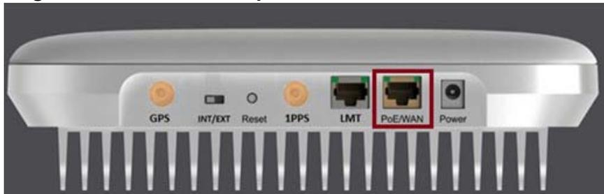
[Table 2-1](#) provides the recommended PoE specifications for the Network Extender.
