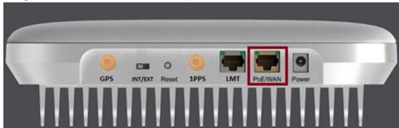
4. Connect the other end of the Ethernet cable to a port on the home router/switch or connect it to the Ethernet outlet that has service.
