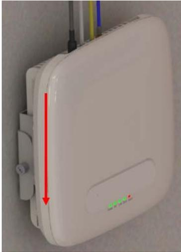
4. Tighten the screw fasteners, one on each side (see [Figure 2-7](#)).
