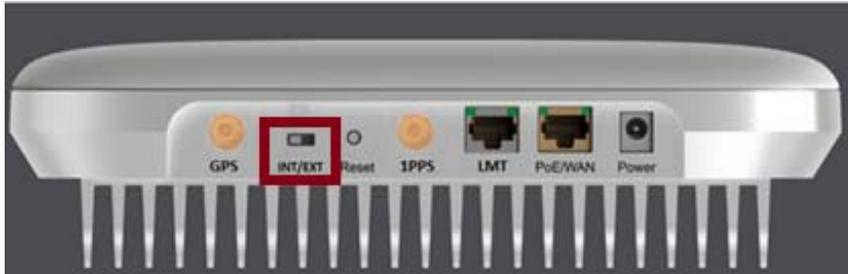
Setting the Network Extender to EXT without an external antenna connected will end with PA damage. Changing the switch during unit operation produces the same effect.
