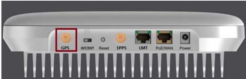
2. Position the GPS antenna puck near a window so it provides a clear and open view of the sky.
