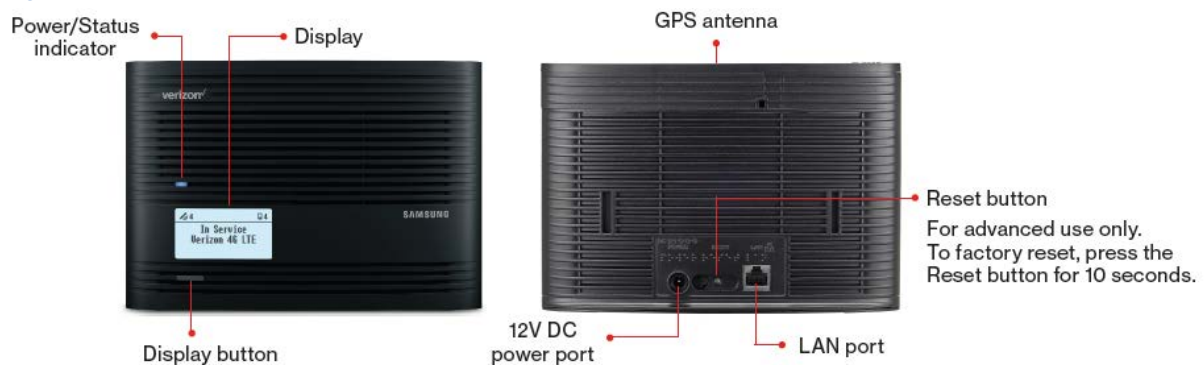
Figure 4. Components - Front and Rear View
