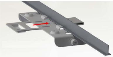
**3.** Push the clamp back against the T-Rail to engage tabs on both sides of the rail (see Figure 2-10).
