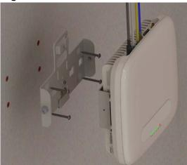
2. Align the tabs on the upper bracket with the opening on the lower bracket and push inward (see Figure 2-5).
