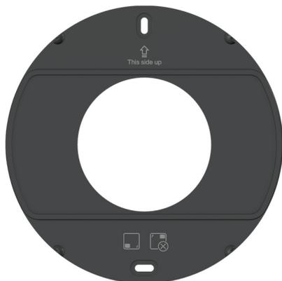
1. Screw the included wall mount bracket into desired position on a wall securely, ensuring it's the correct way up (screws are included with the wall-mount). Recommended hole size for the conical plastic anchor is 0.25" in diameter and 1.20" in depth.
