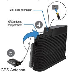
**Warning!:** Do not force the connector into the GPS antenna port as this can damage the connector.
