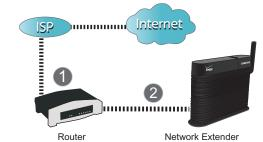
Connect one end of the included Ethernet cable to an open LAN port on the router (1) and connect the other end to the WAN port located at the rear of the Network Extender (2).
