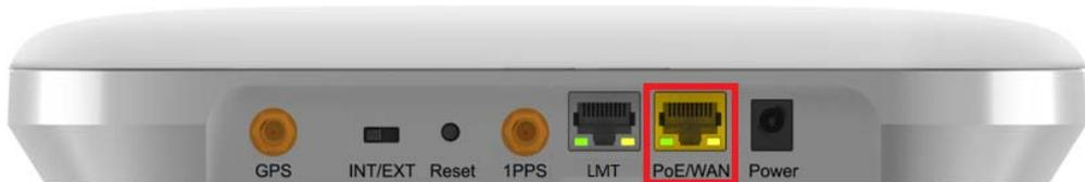
[Table 2-1](#) provides the recommended PoE specifications for the Network Extender.
