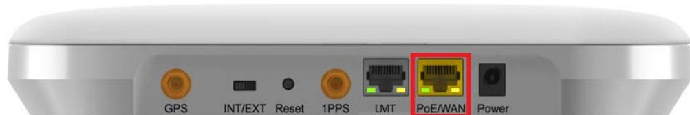
4. Connect the other end of the Ethernet cable to a port on the home router/switch or connect it to the Ethernet outlet that has service.
