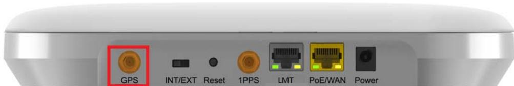
2. Position the GPS antenna puck near a window so it provides a clear and open view of the sky.
