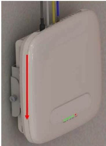
4. Tighten the screw fasteners, one on each side (see [Figure 2-7](#)).
