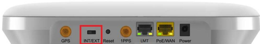
Setting the Network Extender to EXT without an external antenna connected will end with PA damage. Changing the switch during unit operation produces the same effect.
