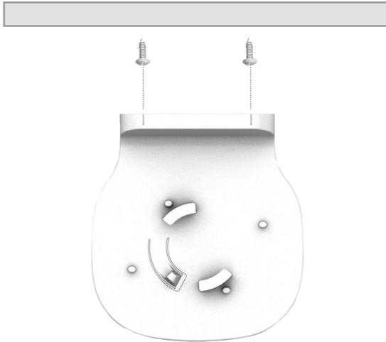
5. There are two mounting slots located on the bottom of the Fios Home Router. It allows you to securely attach your router to the wall. Align the slots with the wall mount bracket.
